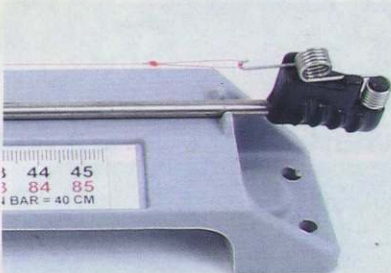
1 Longer than 45cm - Set the boom to e.g. 50cm, hook the loop onto the spring.
